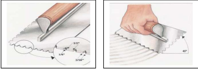
**Note:** Change the trowel every 2,000 to 3,000 SF due to wear down of the notches. This assures the proper spread of adhesive.
